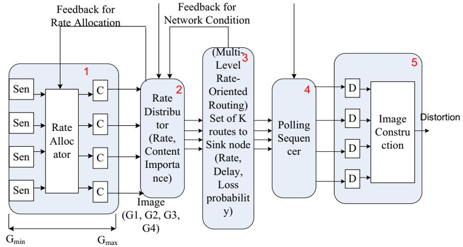
Fig. 1. Architecture design for image transmission utilizing both region and path diversities
