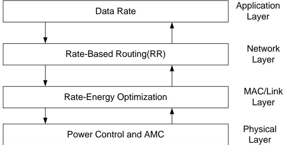
Fig. 2. Network layer Protocol architecture
