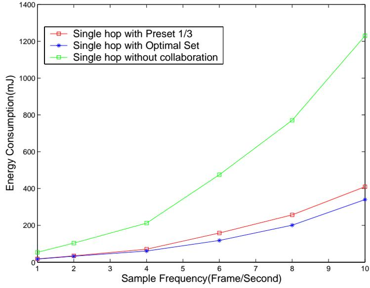
Fig. 4. Energy Consumption Vs Sampling Frequency
