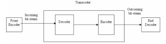
Figure 2. A typical transcoder architecture
