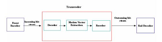
Figure 3. General scheme for motion vector reuse transcoding
