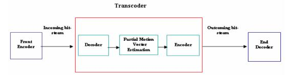
Figure 4. video transcoding scheme for partial motion vector estimation
