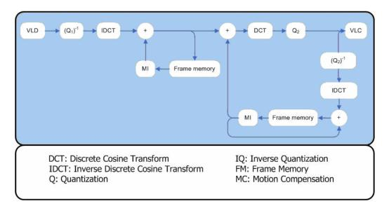
Figure 7. Cascaded pixel domain transcoder
