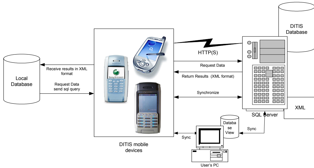
Figure 7. DITIS mobile system architecture
