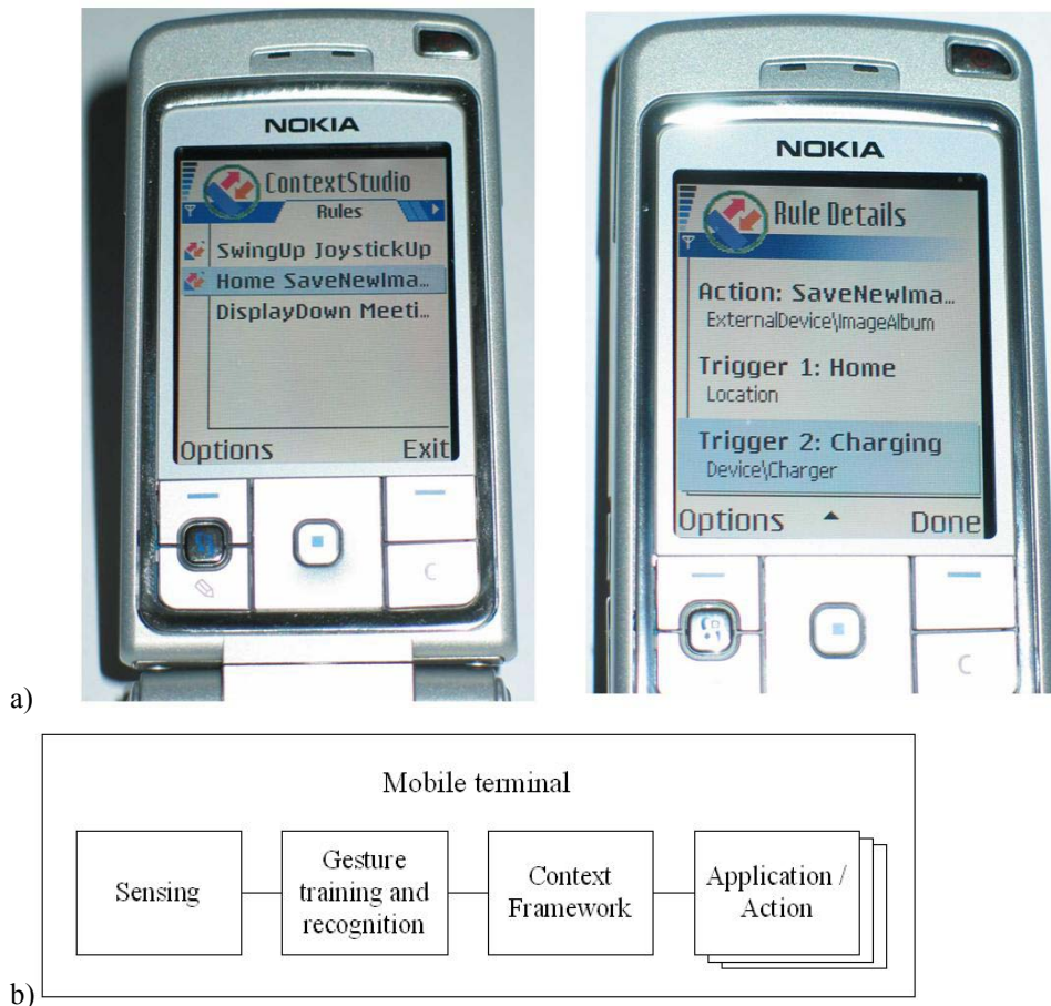
Figure 3. a) Examples of user interfaces, and b) a conceptual overview of a personal device gesture control system
