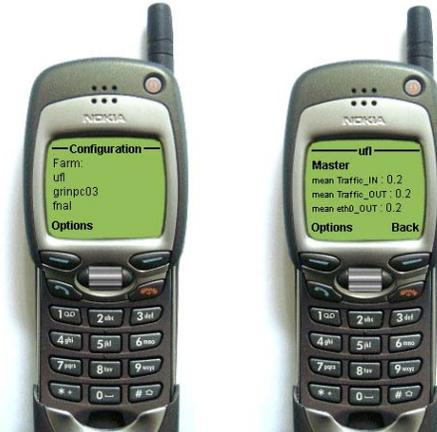
Figure 8. *Mini client: WAP enabled mobile phone: WML content*
