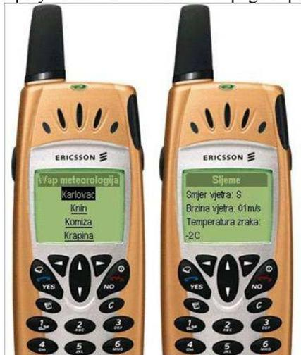
Figure 11. Mini client display: WML
