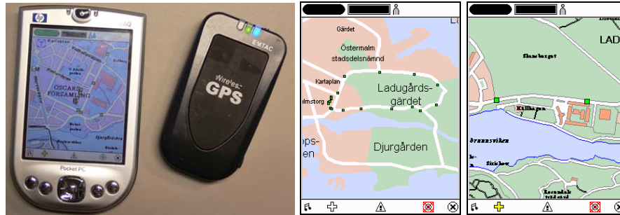
Figure 2. An HP Ipaq 4150 PDA and a Bluetooth GPS Receiver (a). Screen shots of Road Talk. (b) Map show zoom level 1 (b) and level 2 (c) centred on the same coordinate. The squares indicate locations of memos.
