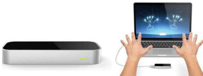
Figure 3 Appearance and principle of operation of the Leap Motion controller [29].
