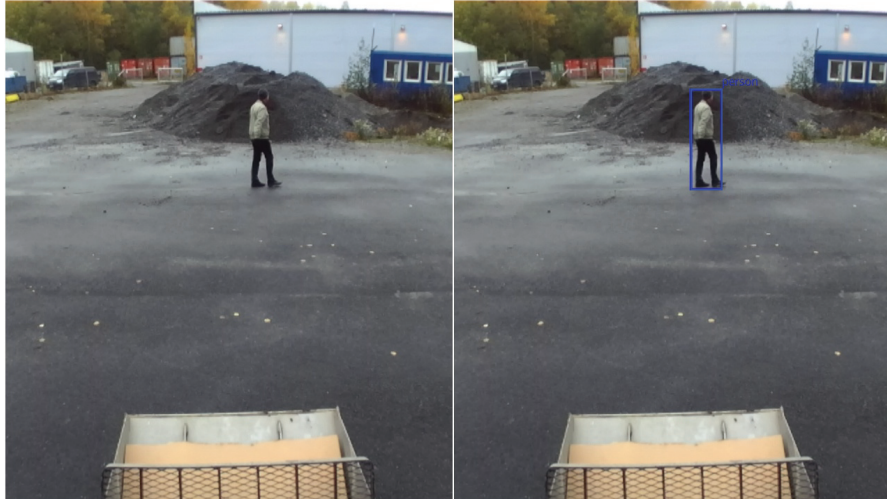
Figure 4 Image captured from the video of the industrial vehicle for which object detection using service based inference and service orchestration is studied. On the left the original image and on the right the object detection output with a bounding box.
