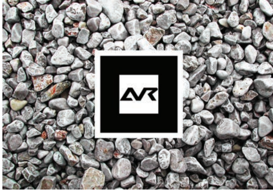
Figure 4 Marker object used in our sequences. The fiducial marker in the center has side s = 7\text{cm} , while the entire texture has dimension 24,7\text{ cm} \times 17,3\text{ cm} .
