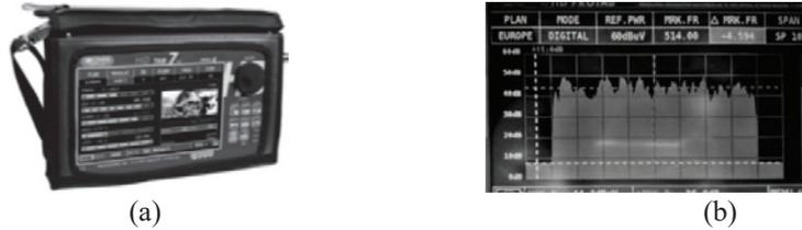
**Figure 12** Measurement equipment (a) DVB-T2 analyzer (b) Example spectrum mask of MUX 1.
