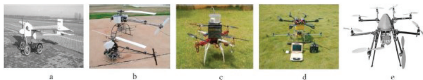
Figure 6 Types of Unmanned Aerial Vehicle (UAV) (a) Fixed Wing (b) Single Rotor (c) Quad Copter (d) Hexa Copter (e) Octo Copter.
