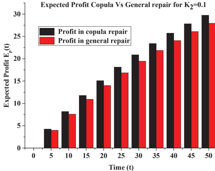
**Figure 8** Comparison in expected profit for copula Vs general repair for  $K_2 = 0.1$ .
