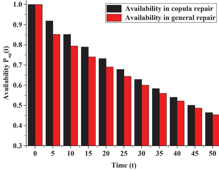
**Figure 2** Comparison in availabilities w.r.t time under different repair policies.
