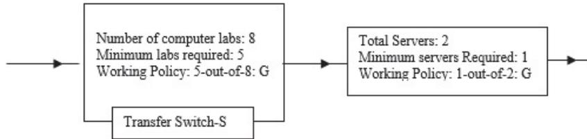
Figure 1(a) System configuration of the model.
