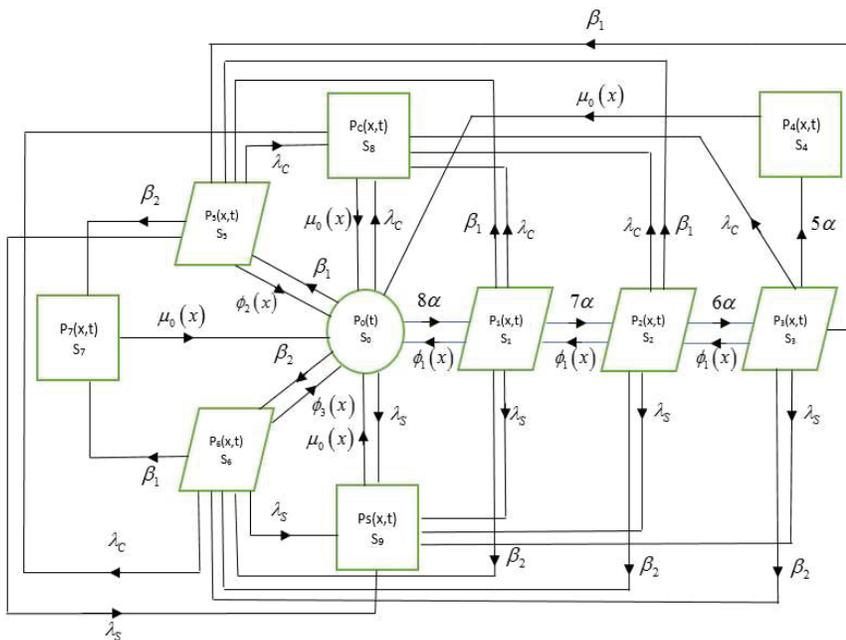
Figure 1(b) State transition diagram of the model.
