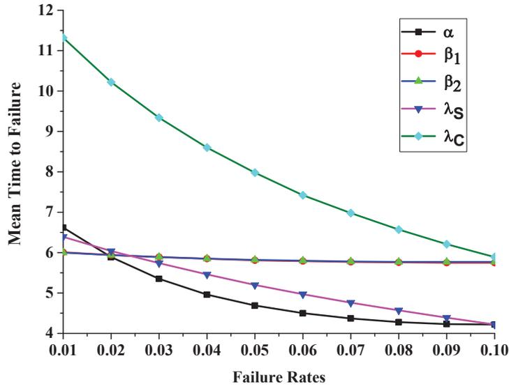
Figure 4 MTTF as a function of failure rates.
