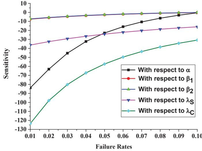
Figure 5 Variation in sensitivity in MTTF corresponding to failure rates.
