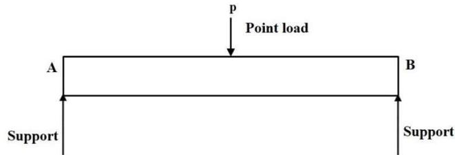
Figure 2 Simply supported beam subjected to the point load at midpoint of span.
