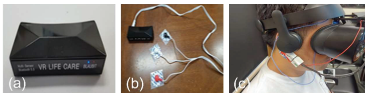
Figure 6 Composite biometric sensor terminals with EEG and PPG(photoplethysmography) data extraction and transmission functions. (a) sensor device 1; (b) sensor device 2; (c) sensor head mounting device.
