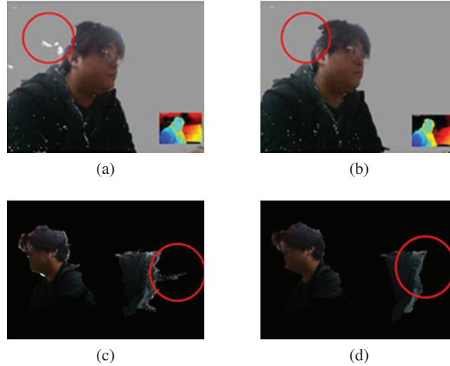
Figure 14 Geometric enhancement result (a) noise caused by lighting, (b) noise reduction result, (c) noise due to unclear boundaries, (d) noise reduction result.
