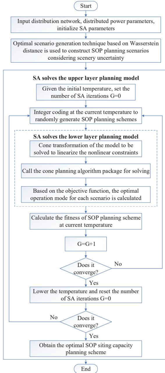
**Figure 2** Flowchart showing the SOP's optimal siting and sizing.
