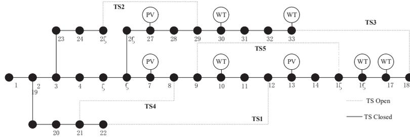
Figure 3 Structure of the IEEE 33-node test feeder.
