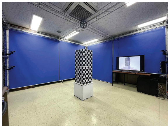
Figure 10 Built experimental environment for capturing the 3D object.
