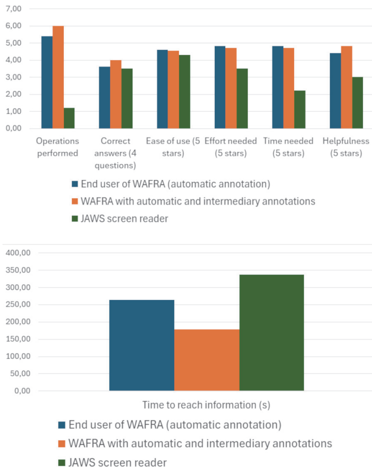
Figure 12 Summary of the experiment with mean values of users' results, including users of WAFRA with automatic annotations only, users of WAFRA with both automatic and manual annotations and users of a screen reader (JAWS).
