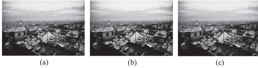
Figure 13 Results of applying noise removal filters to salt-and-pepper noise-added images: (a) Gaussian filter, (b) median filter, (c) BM3D.
