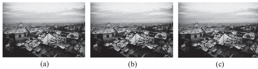
Figure 12 Results of applying noise removal filters to Gaussian noise-added images: (a) Gaussian filter, (b) median filter, (c) BM3D.
