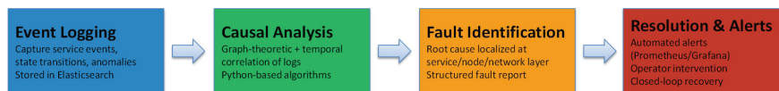
Figure 7 Diagram illustrating the fault localization process, from event logging to root cause identification.
