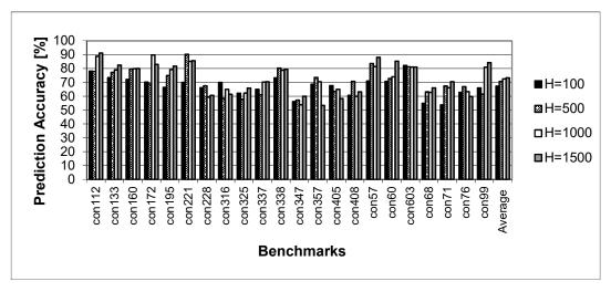
Figure 7. Prediction accuracies obtained with the DDT-M1-4 predictor using different link history lengths
