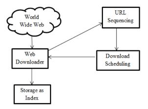
Figure 2 Typical Web Crawler System architecture.
