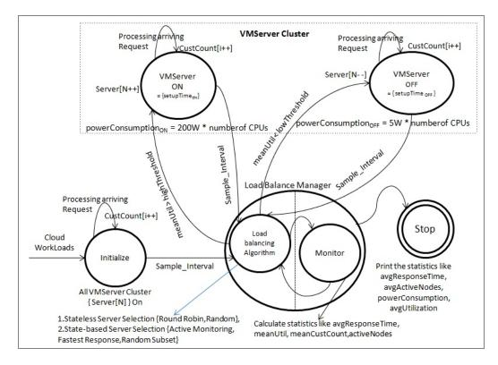
Figure 1 The state transition diagram of the performance constrained power management policy for various load balancing algorithms for the cloud.
