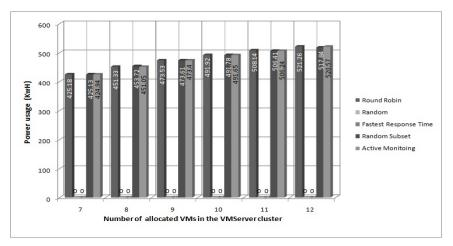
Figure 3 Power usage comparisons of stateful and stateless load balancing algorithms for single core VMs.
