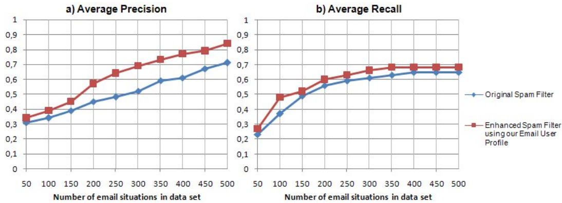
Figure 5 - Comparative performance of email filtering with and without personalization (a) Average precision with different number of email situations. (b) Average recall with different number of email situations
