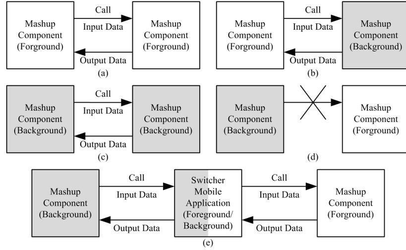
Fig. 8. Conventional inter-application protocols are shown in (a) to (c) where (d) is not permitted. A SMA-based inter-application protocol (shown in(e)) enables an indirect communication between a call from a background process to a foreground process
