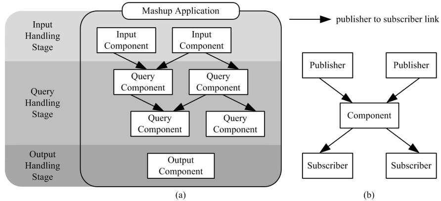
Fig. 4. Abstract data flow model. (a) shared tree model of a mashup application and (b) direction of data flow of a component with its publishers and subscribers.
