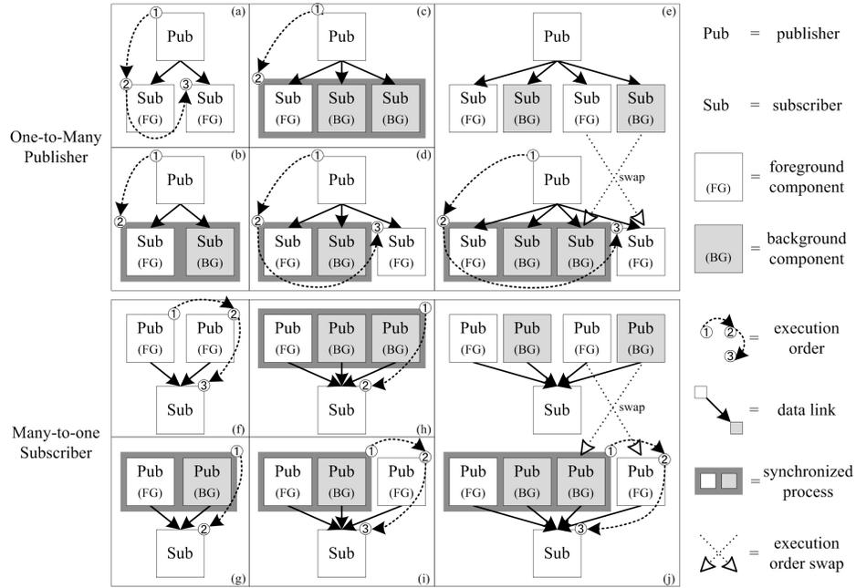
Fig. 10. Process Synchronization in the second phase of Mashup Process Scheduling Mechanism.
