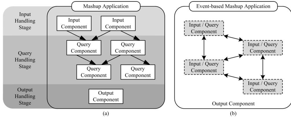
Fig. 16. The comparison between flow-based and event-based mashups. (a) In flow-based mashups, the execution order follows the top-down shared three models of data and control flow. The output is generated and displayed in the last order. (b) In event-based mashups, the contained components communicate with each other in back-ground processes by handling the input/output events. The output display is updated in real-time executions of the integrated components.
