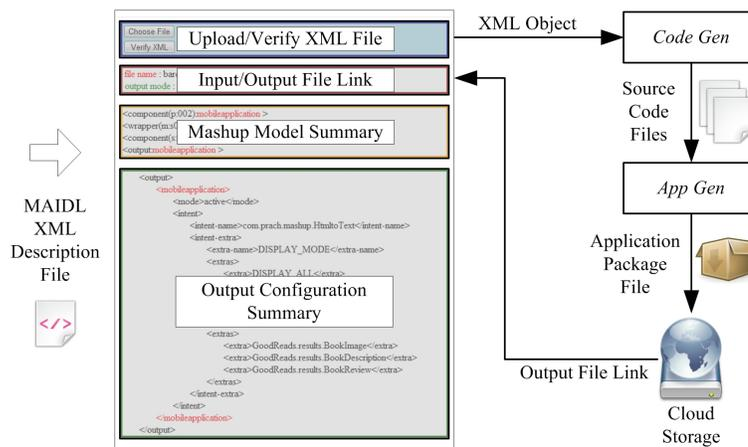
Fig. 7. Workflows of *Code Gen* and *App Gen* Module in the generation phase.
