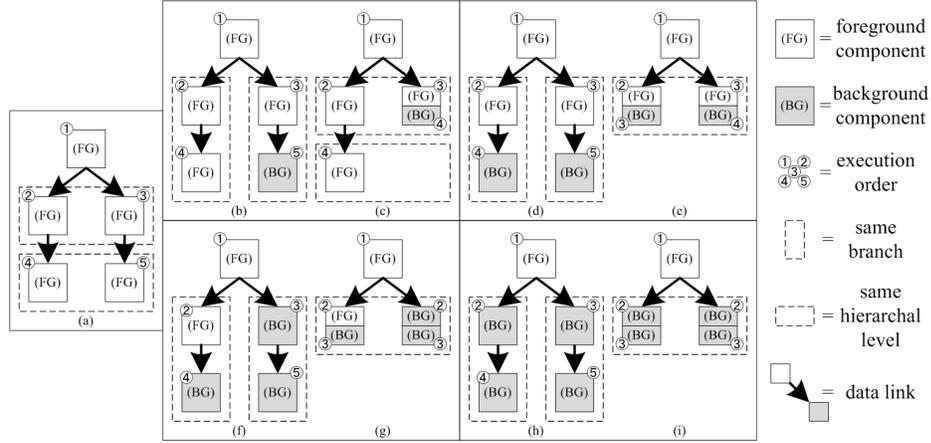
Fig. 9. Tree Level Reduction in the first phase of Mashup Process Scheduling Mechanism.
