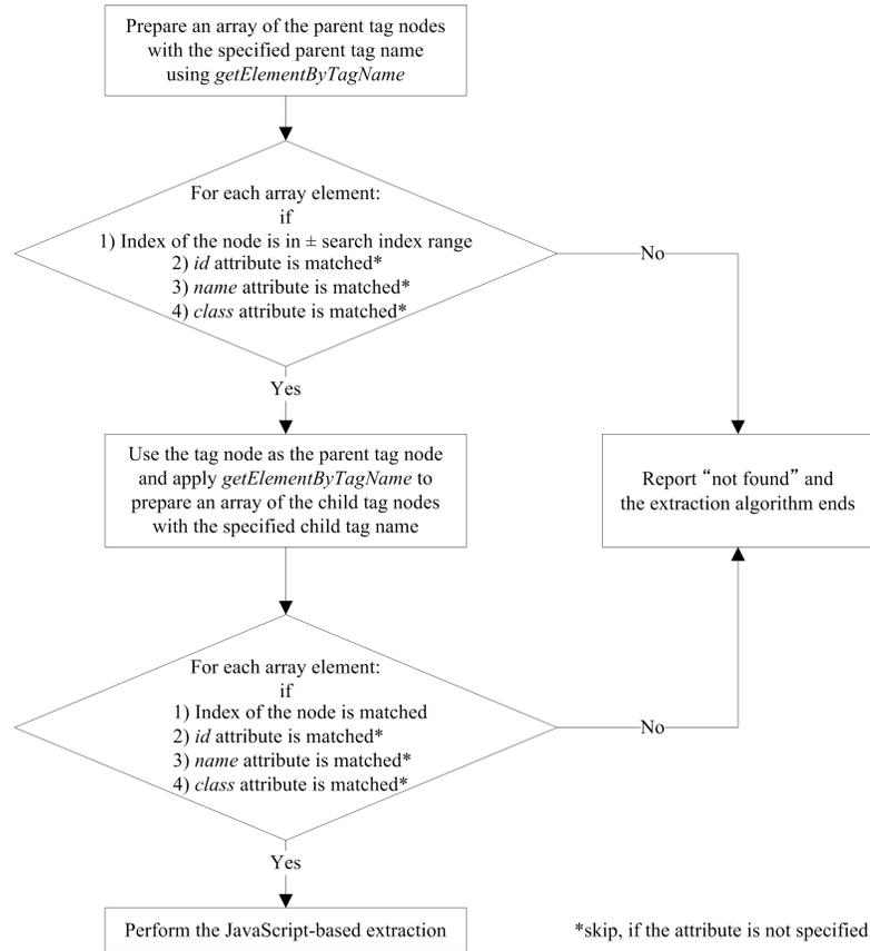
Fig. 3. Extraction algorithm used in Web application component.
