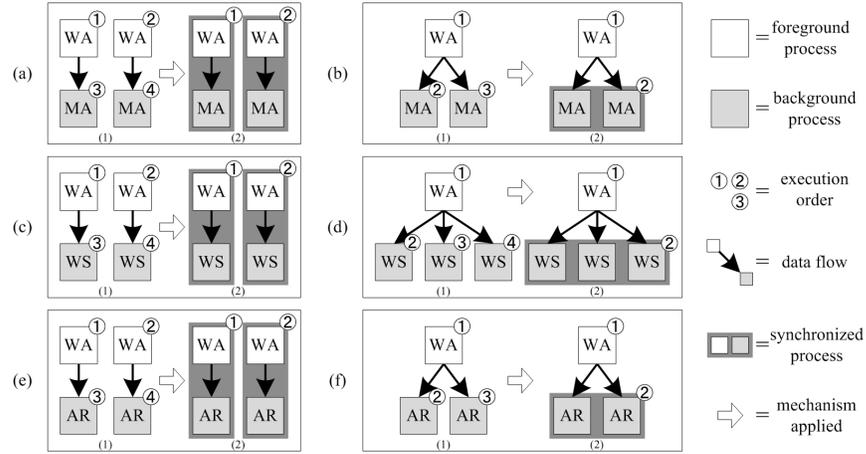
Fig. 13. The Model of Mashup Example used in Performance Evaluation. (a),(c) and (d) applied the first phase of the *Mashup Process Scheduling Mechanism*. (b), (d) and (f) applied the second phase of the mechanism. In (a) and (b), we use Amazon WA component, and database MA component. In (c) and (d), we use Amazon WA component and ExchangeRate WS component. In (e) and (f) we use Wikipedia WA component, and AR component that calculate GPS distance.
