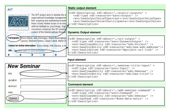
Figure 4 Examples of the atomic user interface elements and their RDF definitions.
