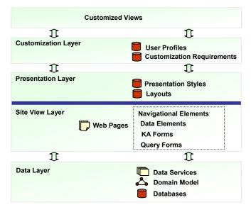
Figure 1 The extended architecture of data-intensive web sites.
