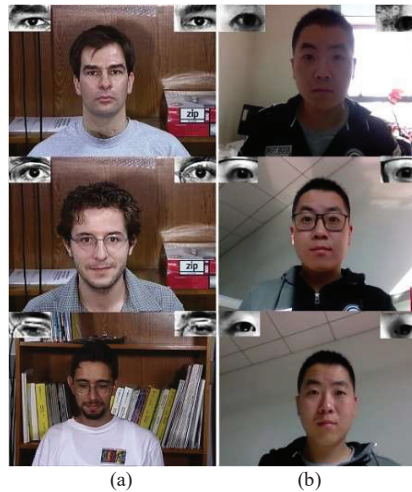
Figure 7 Eye region detection result: (a) images from the Georgia Tech face database [10] and (b) images during actual use.
