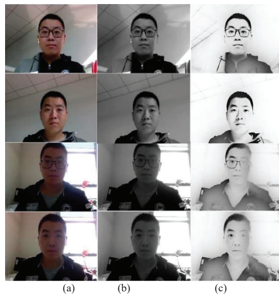
Figure 4 Use of LSH to remove the effects of illumination(author): (a) original image, (b) grayscale image, and (c) LSH result.
