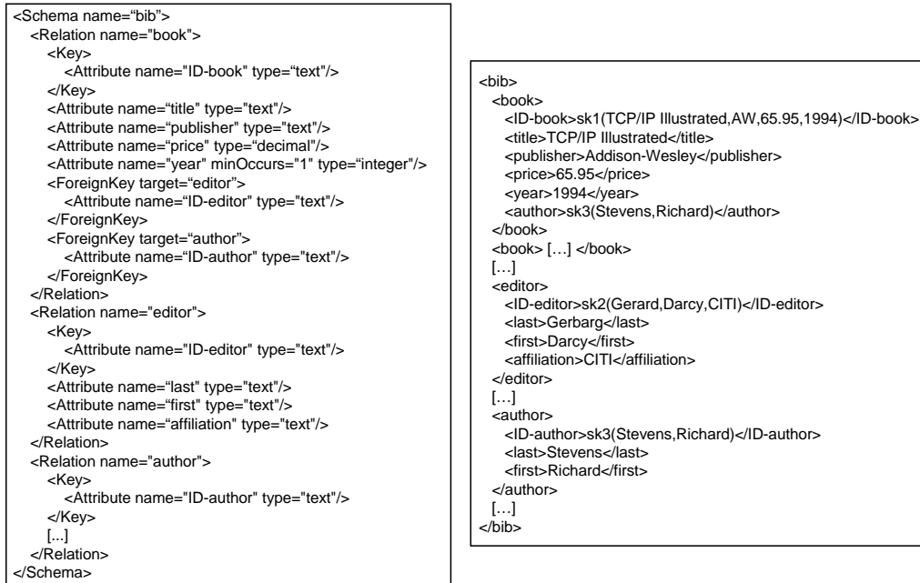
Fig. 7. The target data of the second translation and the corresponding scheme in relational format
