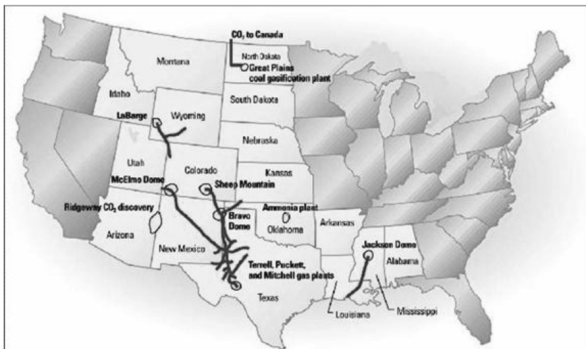
Figure 5. Carbon dioxide sources and pipelines serving enhanced oil recovery projects in the United States.
