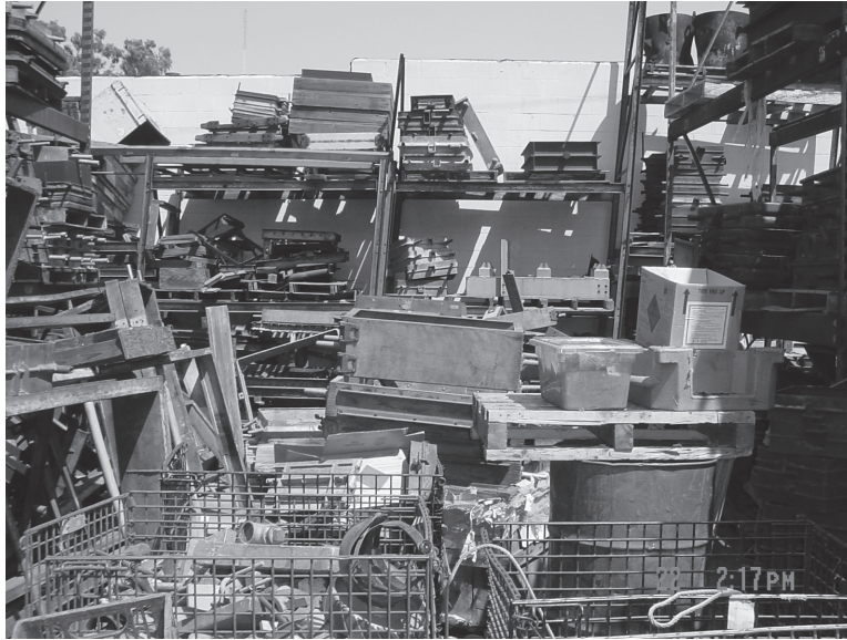
Figure 2. In this messy plant the workers waste close to 20 percent of their time looking for items and scavenging for parts and tools, also wasting the plant energy.
