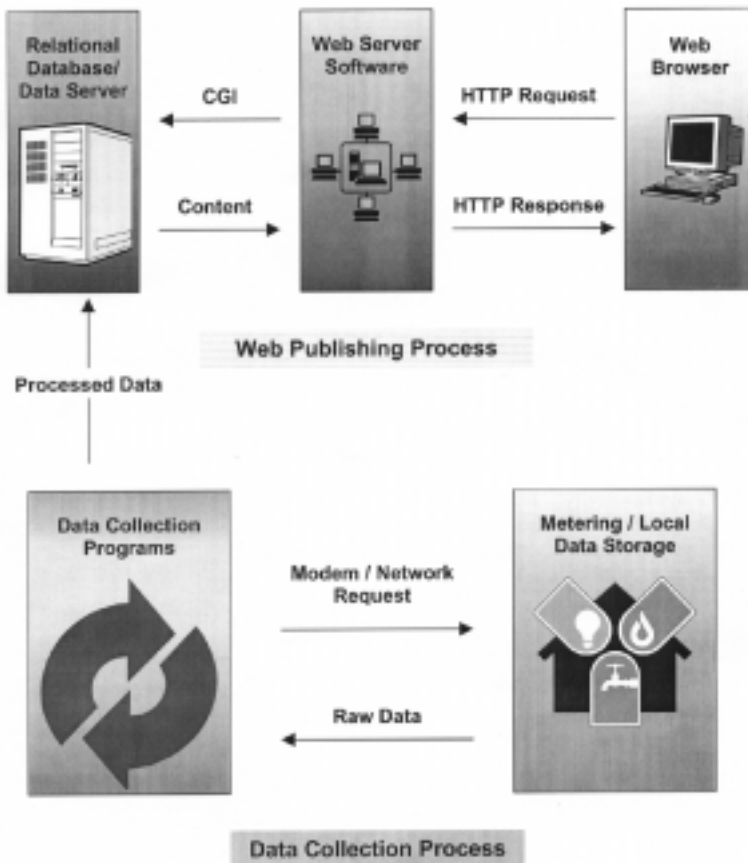
Figure 1. Energy Information System Functional Layout
