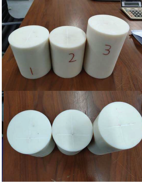
Figure 12 3D printing of full-diameter core samples of white resin with caves NO. 1, NO. 2 and NO. 3.
