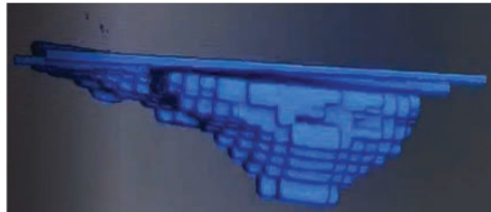
Figure 16 Reconstruction map of CT scanning results for NO.3 cave.
