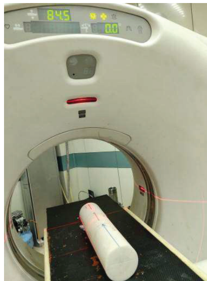
Figure 13 CT detection of 3D-printing full diameter cores.
