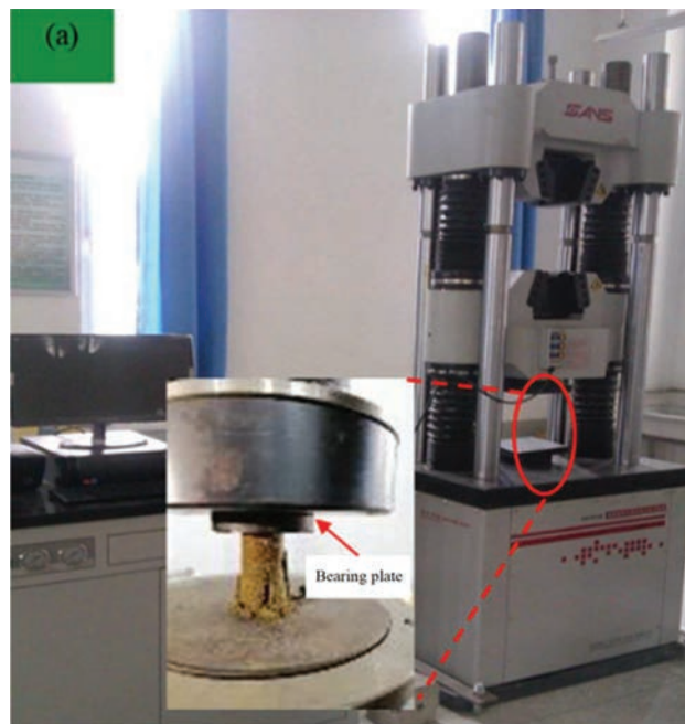
Figure 11 Rock mechanics testing equipment—SHT-4106 material testing machine.
