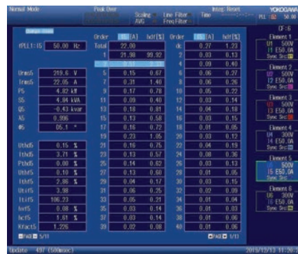
Figure 8 Statistical analysis with f = 50.00 Hz.
