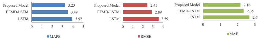
Figure 9 MAPE (%), RMSE (W/m 2 ) and MAE (W/m 2 ) of developed models on an annual average basis.
