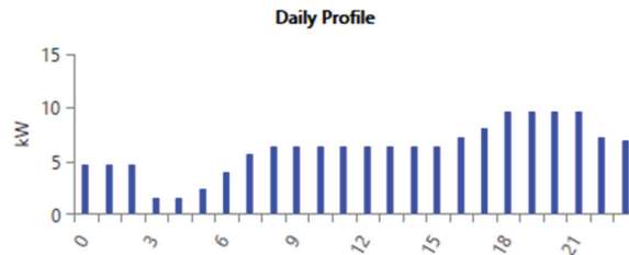
Figure 5 Electric load of a house with an Electric vehicle.
